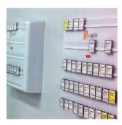
The vertical high-density storage system, equipped with drawers that can easily be pulled out to access their contents, provides an organized system, making it easy to locate supplies. It also maximizes the capacity of the storage footprint.
